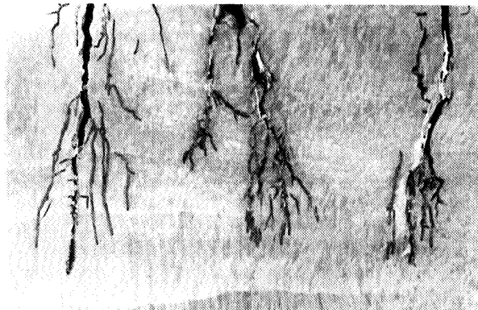
Figure 8. A photomacrograph of the inner portion of a longitudinal section of the weld in the 7-in. sample, illustrating the branching crack patterns. (Oxalic acid, electrolytic etch. 5X.)
